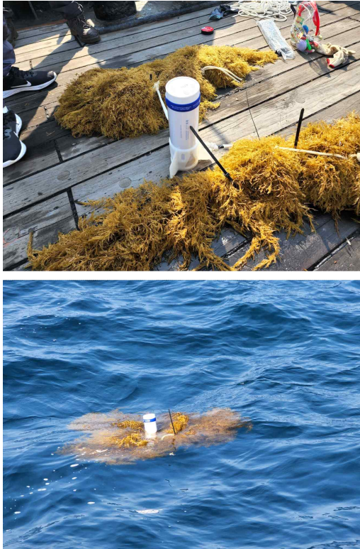
Figure 6. Attachment example between sargassum and drifters. The top picture shows connecting the sargassum to the buoy, and the bottom image indicates the linked sample floating in the ocean
